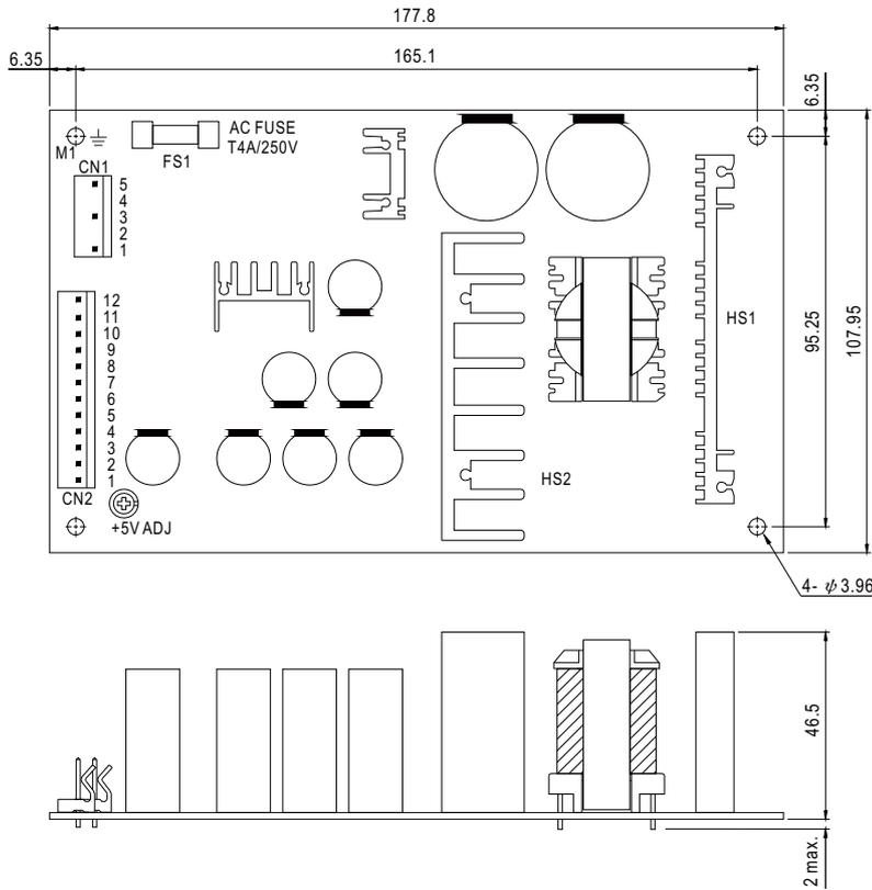
AC Input Connector (CN1) : Molex 5273-05 or equivalent
